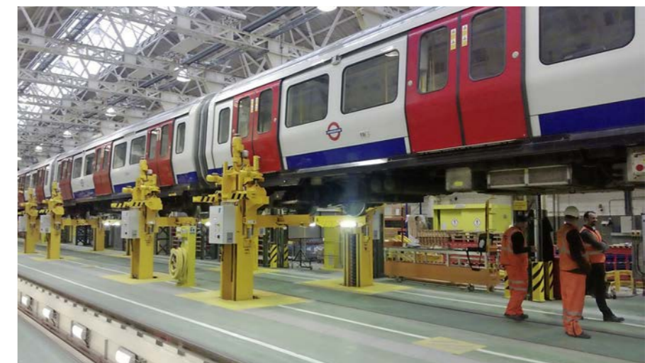
New hydraulic jacks at Upminster depot can lift an entire S-Stock train. TAYLOR WOODROW.
