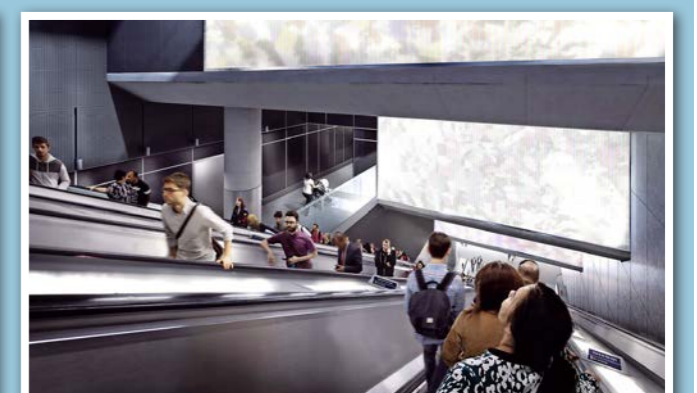
The escalators leading down from Dean Street (western) ticket hall. Above them, a sequence of screens will display digital artworks by Turner Prize-winner Douglas Gordon. Weighing 42 tonnes each and being 47m in length, they will be the second longest escalators on the TfL network, as only the escalators at Angel Tube station are longer.
