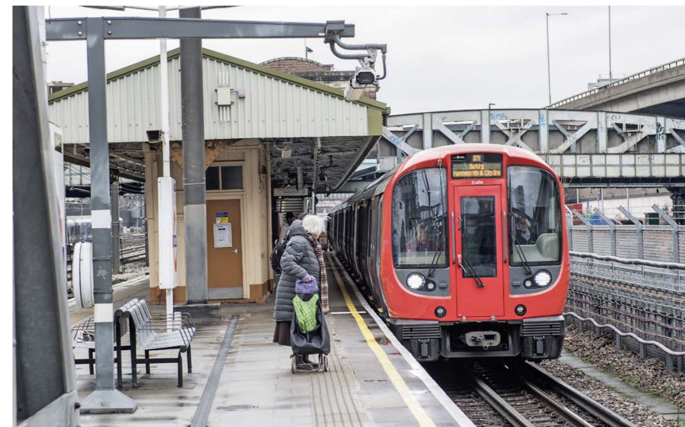
An S-Stock train arrives at Royal Oak on February 2, bound for Barking on the Hammersmith & City Line. The trains were delivered from 2009, and reliability on some sets has reached 200,000 miles per failure. They were the first London Underground trains to be fitted with air-conditioning. JACK BOSKETT/RAIL.
