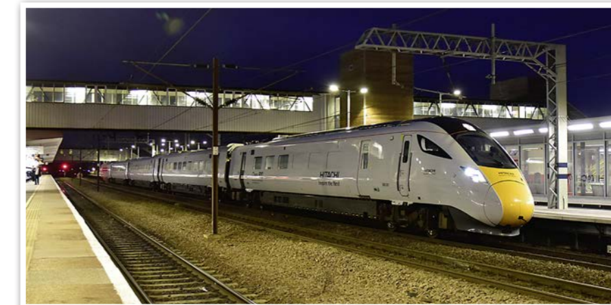
Hitachi Rail Europe bi-mode 800001 stands at Peterborough during a test trip. The Class 800/801s will also enter traffic on the East Coast Main Line from next year, serving London King's Cross as part of the Intercity Express Programme introduction. ALEXANDER CROMARTY.
