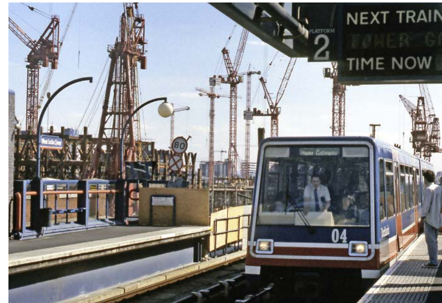
DLR 04 approaches West India Quay on August 18 1989. It is one of DLR's original 11 single-car trains, known as P86 stock. Built by Linke-Hofmann-Busch (now Alstom), the stock was sold and moved to Essen, Germany, in 1991, as the vehicles did not meet safety regulations needed to run in DLR's newly built tunnelled extension to Bank. D. PYE/COLOUR RAIL.
