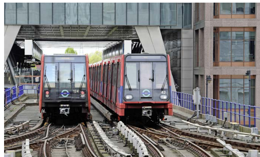
DLR 042 departs Canary Wharf as DLR 124 arrives on April 15 in an image that perfectly illustrates the subtle differences between DLR's Bombardier-built B07 stock that entered service in July 2009 (left), and B90 stock (right) which entered service in 1992. DLR 042 will be withdrawn by 2022, when new rolling stock is scheduled to enter service. PAUL BIGLAND.
