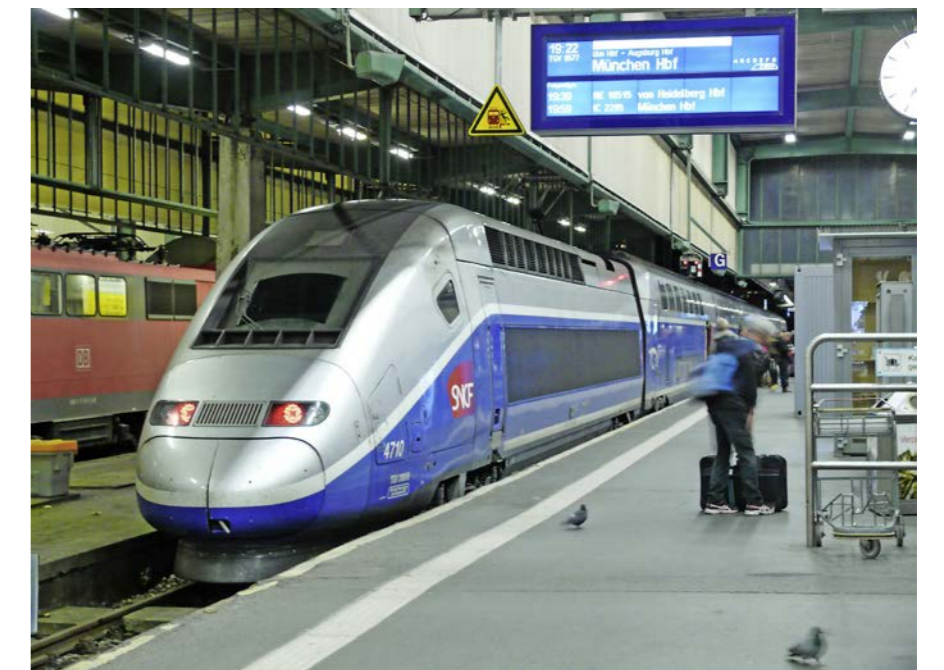
Since the late 1990s, SNCF has focused on building double-deck 'Duplex' TGVs to increase capacity on the busiest routes. On November 27 2016, 'Euroduplex' multi-voltage set 4710 calls at Stuttgart Hbf with a Paris-Munich working. BEN JONES.
