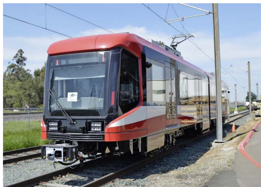
A tram destined for Calgary, Canada, undergoes testing at Siemens' Sacramento factory prior to delivery by rail to the Canadian city.
