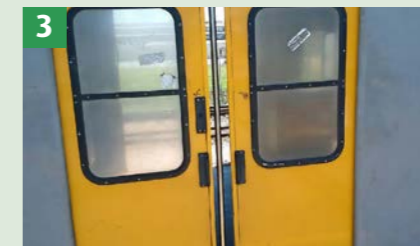
2. A photo of the new train fleet in service. A fault on the new train stock has resulted in the doors opening on the wrong side of the train and exposing the adjacent tracks.
