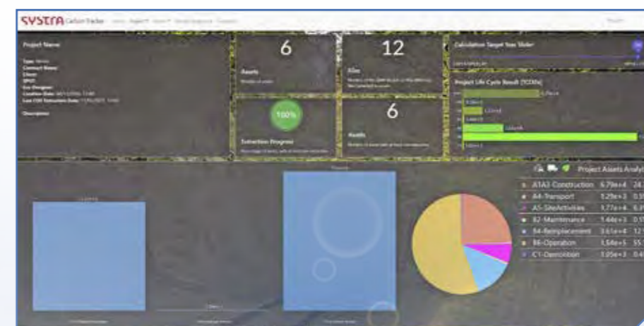
CarbonTracker enables carbon emissions from all stages of the lifecycle of any new piece of infrastructure to be visualised and then benchmarked, so that informed design decisions for lower-carbon alternatives can be made. SYSTRA.
