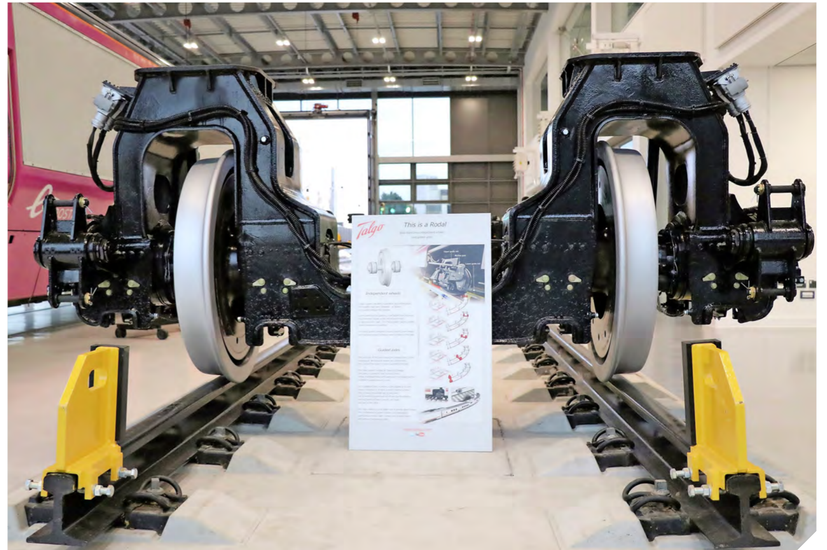
Talgo's Rodal system works by enabling each wheel on an axle to rotate at different speeds, which helps to reduce track wear and tear and lower energy consumption. One has been donated to the National College for Advanced Transport & Infrastructure. TALGO.
