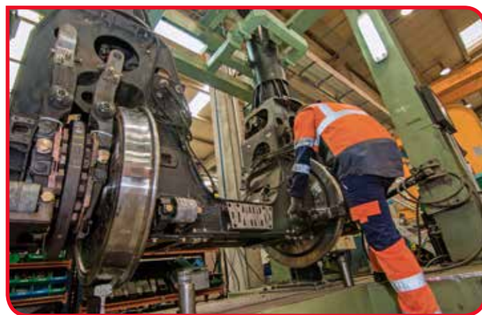
Talgo prides itself on its innovation. Inside the Rivabellosa factory, a member of staff works on a wheelset. Talgo trains are not fitted with axles, but use natural tilt created by their Rodal system to travel around corners on high-speed lines. TALGO.
