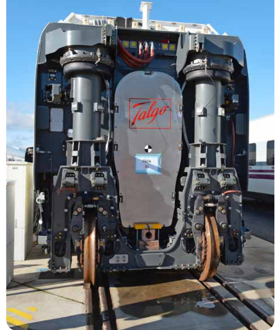
The Rodal wheelset system displayed on a Very High Speed Train set bound for Saudi Arabia. RICHARD CLINNICK.
